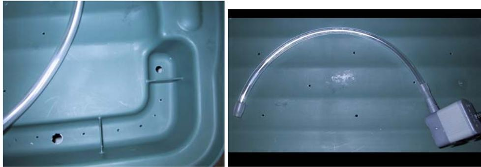
Drill 1 hole large enough for your pump tube and then in a near corner another hole the same size for additional drainage. Assemble your water pump and cut a length of tube long enough to reach from the bottom of the tub to 1" above the hole.
