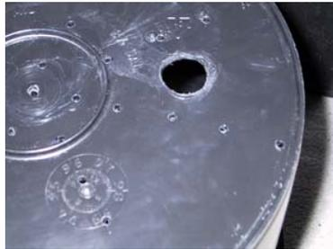
Drill a hole about 7/8" in the 3.5 gal bucket as shown. Your PVC pipe will slide in here.
