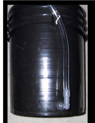
Insert your tube onto the 'L' elbow and carefully slip the elbow into the grommet.
