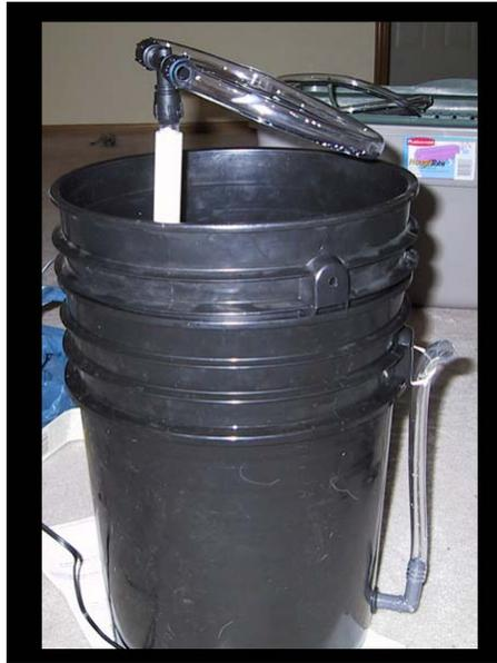
Place the pump in the 5 gal bucket, run the cord carefully out the top.
