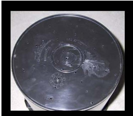
Drill your drain hole in the 5 gal bucket, use the type of drill bit shown for best results. Make certain your drill bit is the right size for the grommet.
