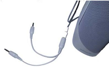
Here is an example of wiring for an automation computer. The stereo jack (this is what you connect the computer speaker output to) below actually is a 3 way splitter providing 6 channels of mono output, the outputs are behind the plate and go to: living room (stereo 2), Entertainment room (stereo2) , Master Bedroom & Bath (mono 1) and garage (mono 1) - 6 total channels.
